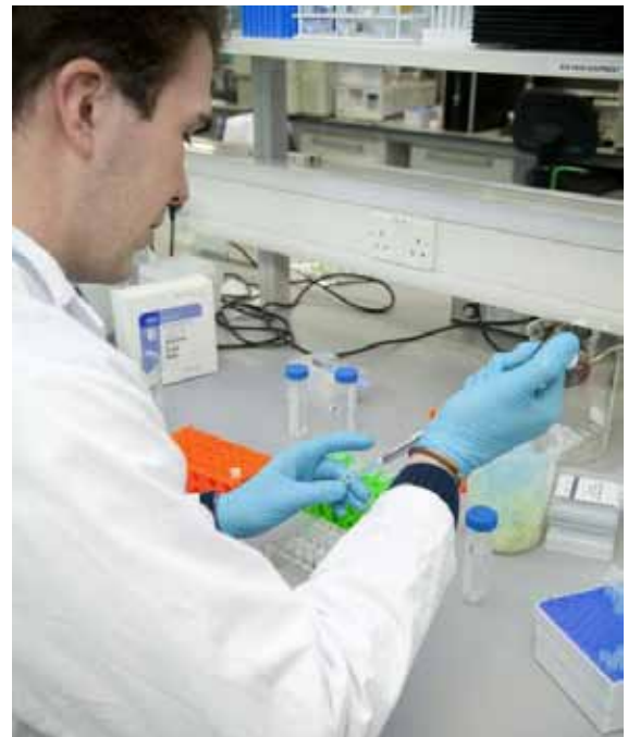
Figure 1: Taking samples from the process for analysis in the plant's lab is the tried-and-true method for ensuring quality control. It's also expensive and not a real-time measurement.
